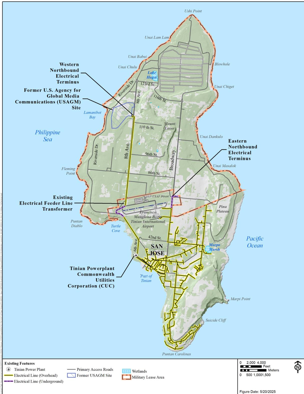
Figure 3. Existing Electrical Distribution System
