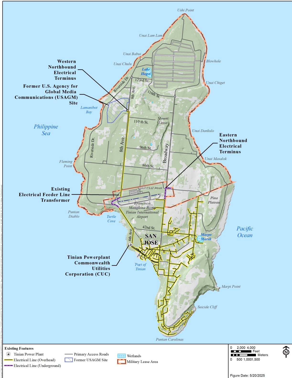
Figure 3 Existing Electrical Distribution System
