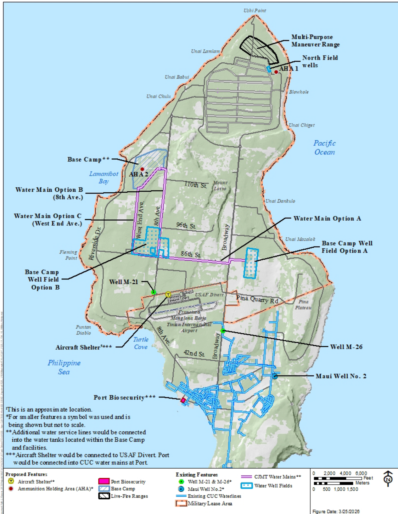
Figure 4.11-1 Water Infrastructure Included in Proposed Action
