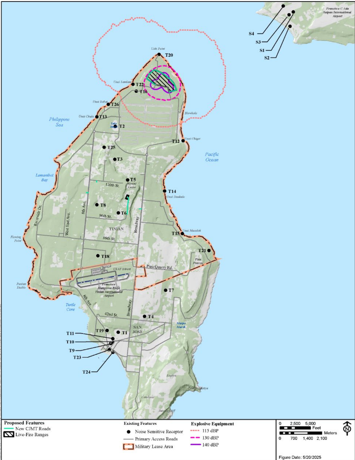
Figure 4.8-2 Peak Sound Levels (Unweighted Decibels) from Typical Explosive Equipment Detonation at the Multi-Purpose Maneuver Range
