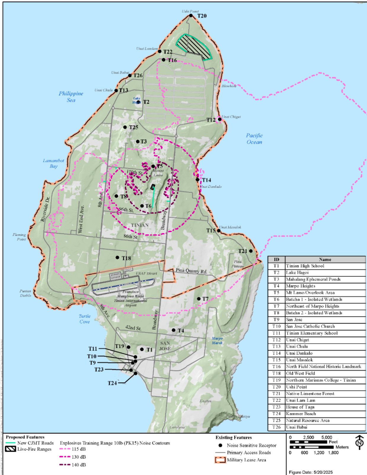
Figure 4.8-4 Peak Sound Levels (Unweighted Decibels) from a 10 Pounds Net Explosive Weight Detonation at the Explosives Training Range
