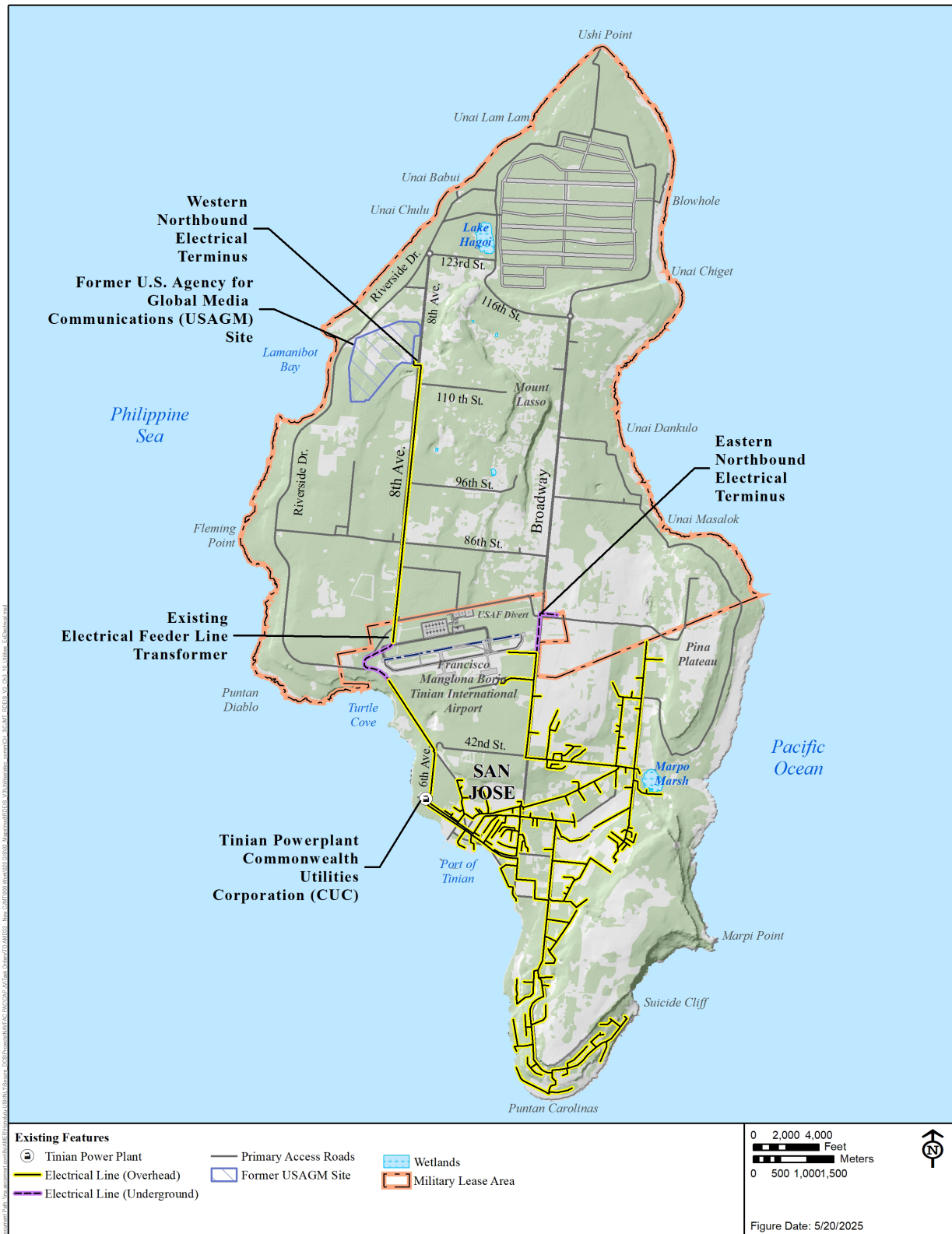
Figure 3 Existing Electrical Distribution System
