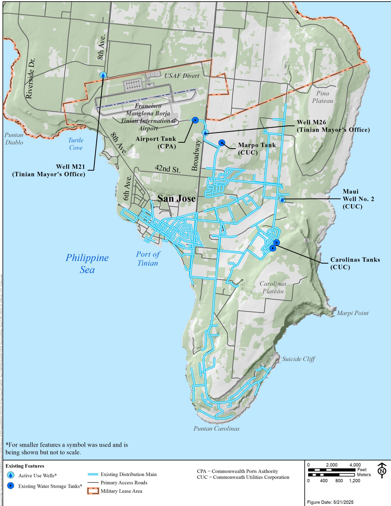
Figure 4 Commonwealth Utilities Corporation Existing Potable Water System
