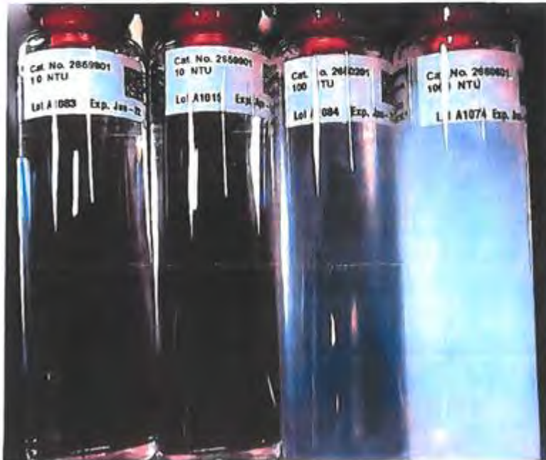
Figure 2 DEQ surveillance laboratory turbidity calibration standards 1.0-1000 NTU
