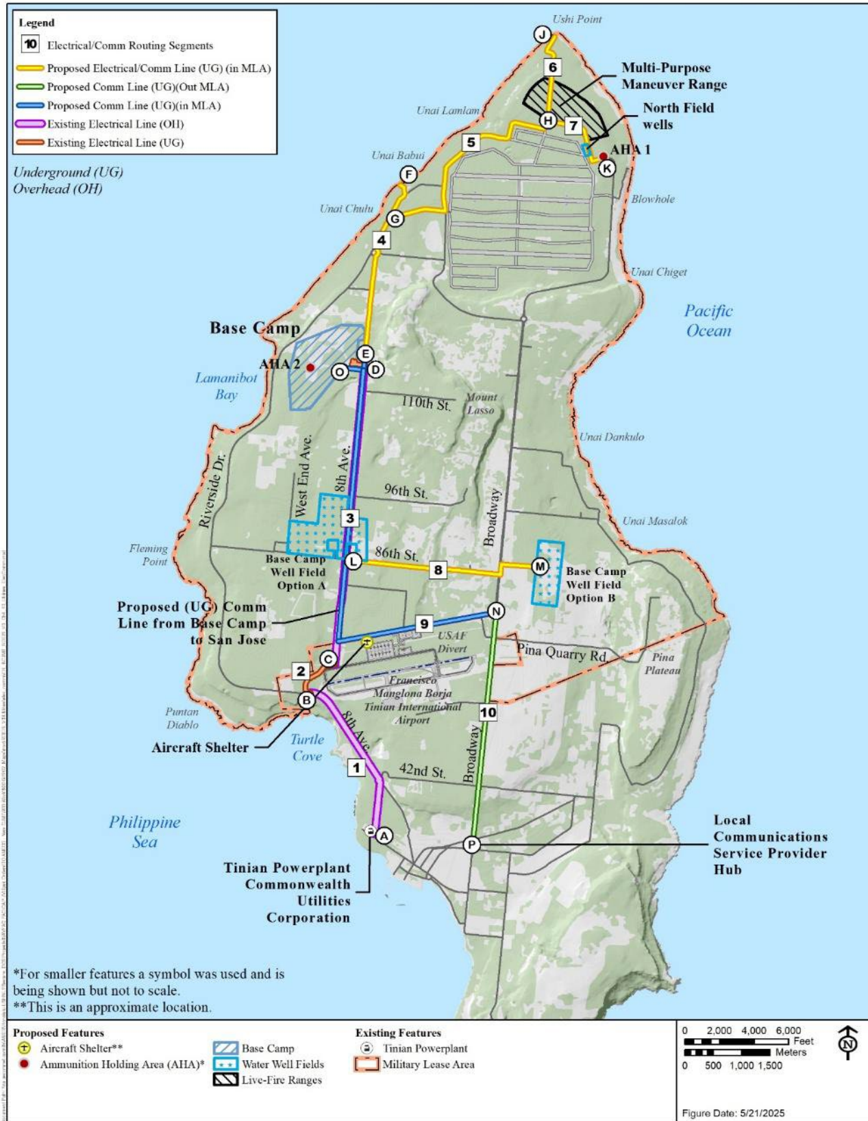
Figure 4.11-2 Electrical Power Distribution for Proposed Action
