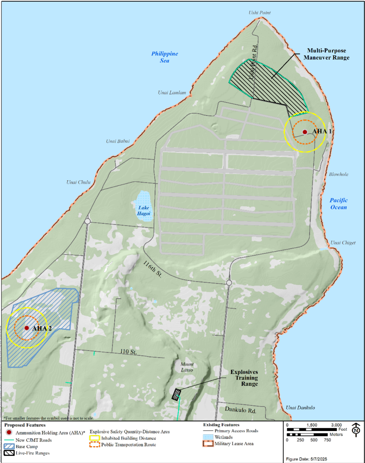
Figure 4.10-2 Ammunition Holding Area Explosive Safety Quantity-Distance Arcs
