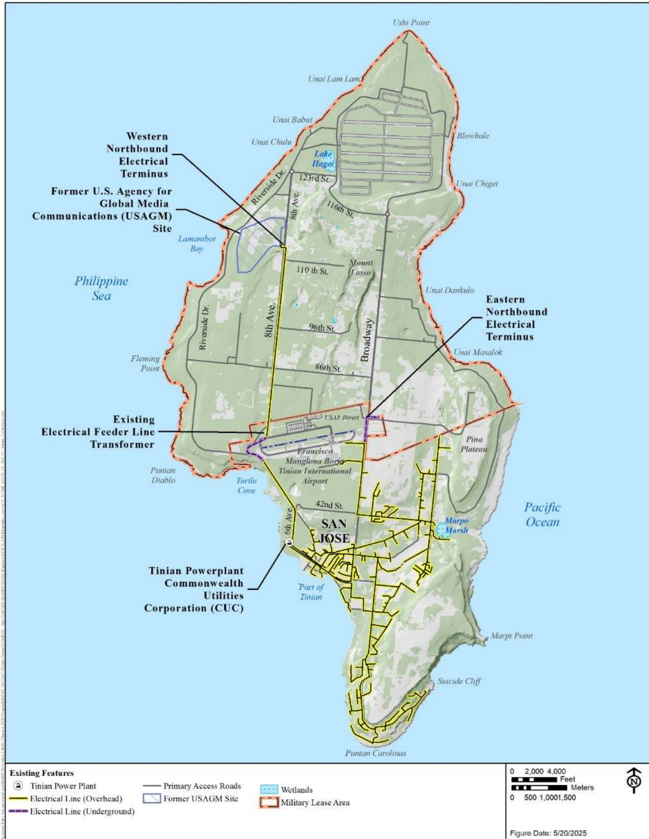
Figure 3.11-2 Tinian Power Distribution
