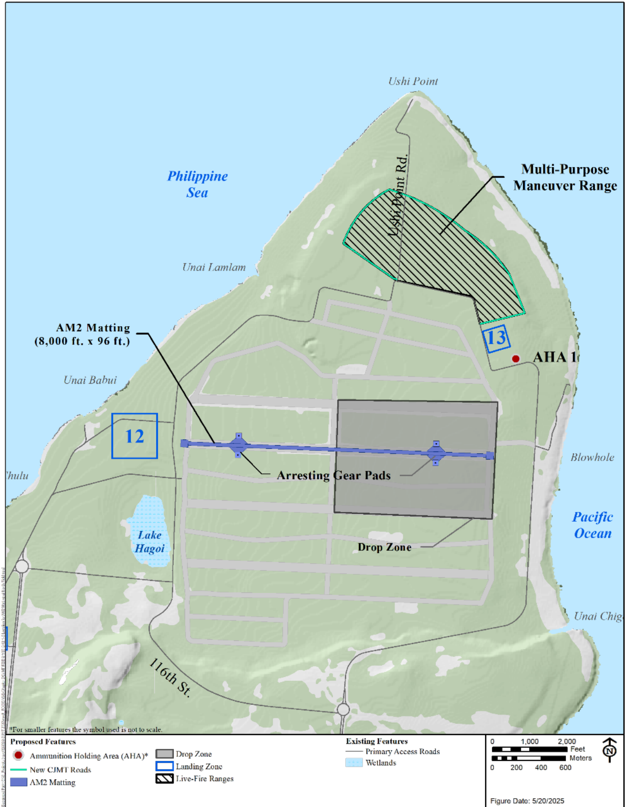
Figure 2.1-5 Location for AM2 Matting at North Field
